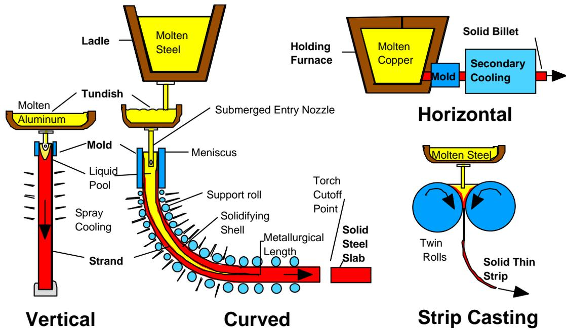
Figure 1. Various continuous casting processes
